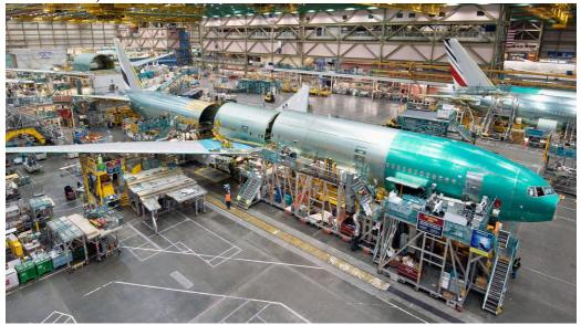
• "The aircraft is then rolled out of the main factory building for the last series of operations: painting of the non-wing exterior surfaces; fueling and fuel systems check; installation and testing of remaining interior items and systems (*e.g.*, in-flight
